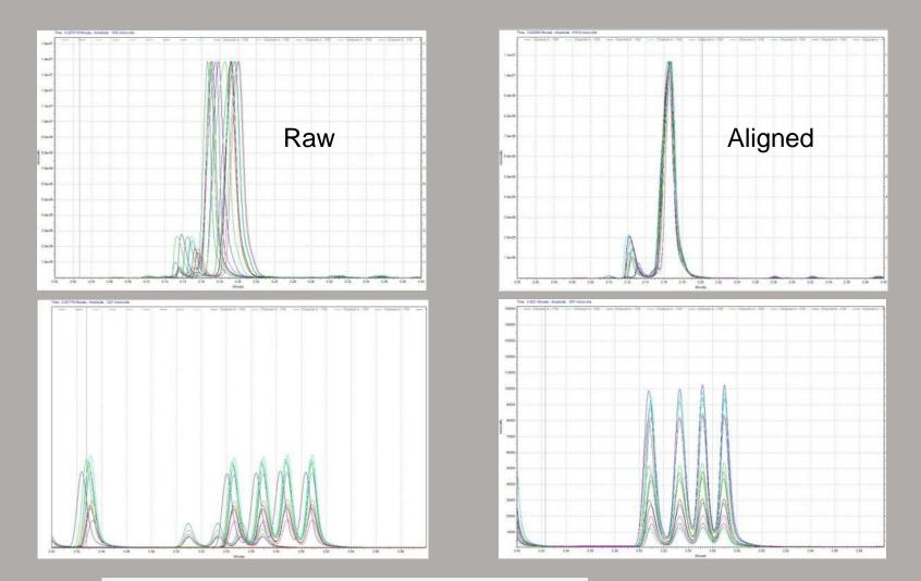
Two instruments with nominally the same method and columns, manual injection
