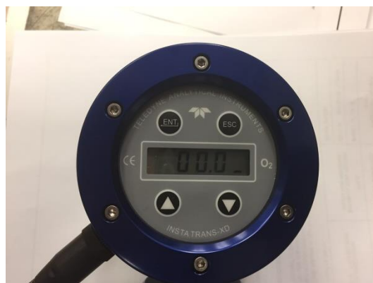
Figure 4-2: Disabled 'No Sens' Warning
